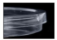
Indented lid is both fully stackable and slippable for use in automated equipment
